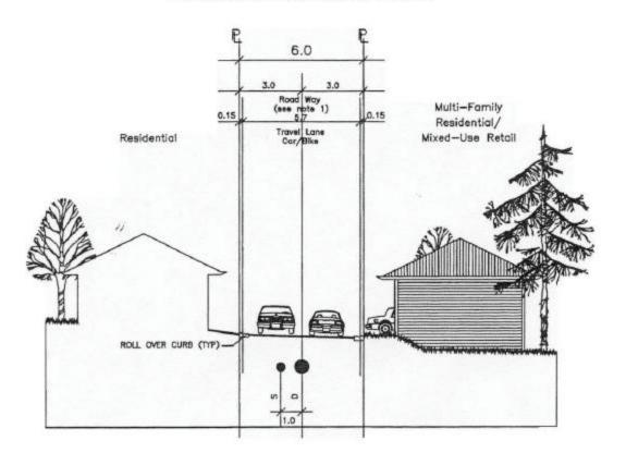
1. WHERE SINGLE FAMILY ABUTS BOTH SIDES, TRAVEL LANE MAY BE REDUCED TO 4.5M. IN THIS CASE, BOULEVARDS MUST BE TREATED WITH A LOW PROFILE, WEED TREE, AUTO ACCESSIBLE SURFACE. THE ROAD GRAVEL BASES TO EXTEND TO FULL WIDTH OF ROW (6.0M).
